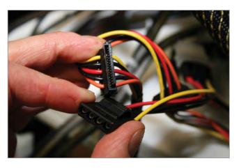
These power supply cables have SATA (top) and 4-pin Molex (bottom) connectors.
