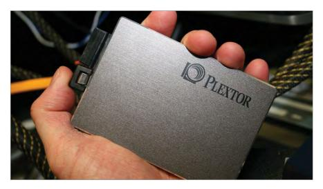
Like notebook hard drives, 2.5-inch SSDs such as this Plextor have different mounting hole patterns than 3.5-inch drives. Since SSDs started to gain popularity, however, some newer cases started to include mounting holes for the smaller drives.
